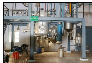
Steam Distillation Unit [700 Liters]
